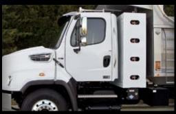
CNG tanks mounted back-of-cab.
